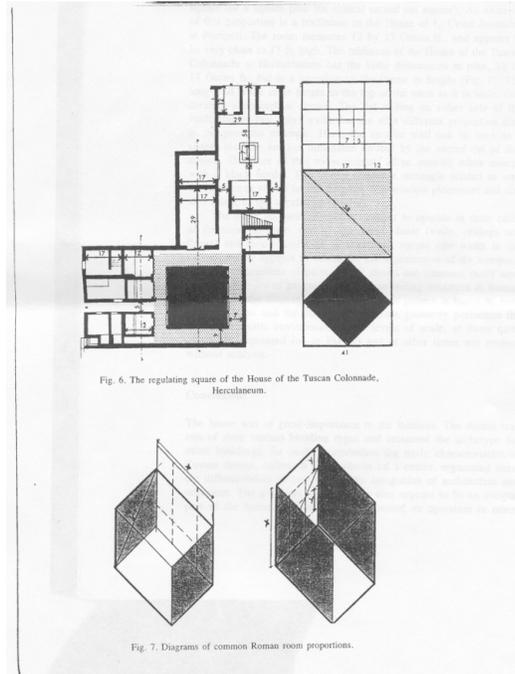
The Watts measure the dimensions in Oscan feet – the Oscans were an early Italic people who built the original walls and towers of Pompeii, and may have founded Herculaneum. As you can see in the floor plan, the Watts found the following dimensions:
