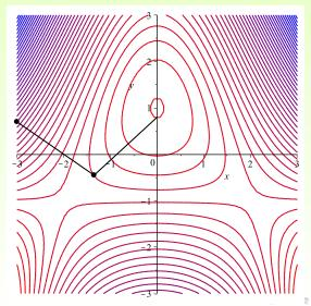
3. Stop. At new point, recalculate gradient.
